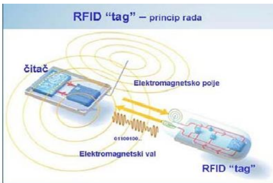
Slika 11.: RFID TAG – Radio frequency identification
