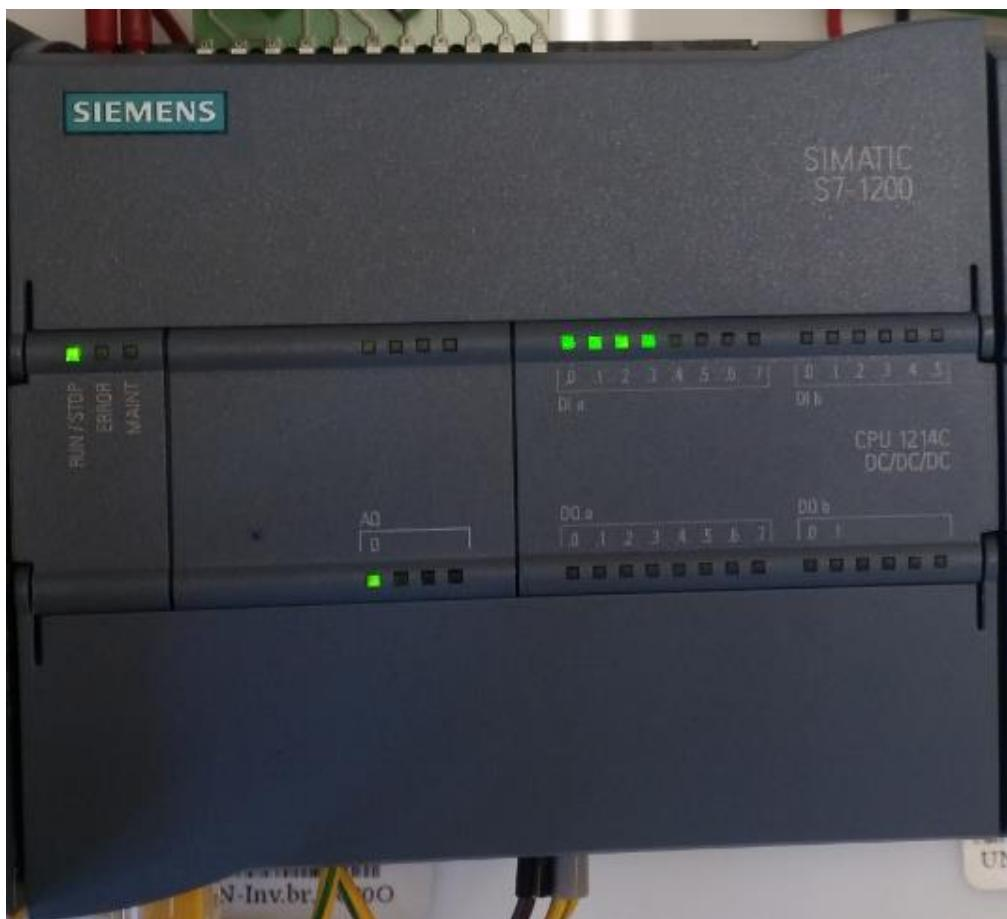
Slika 2.6 Siemens CPU modul S7-1200 - 1214C DC/DC/DC
