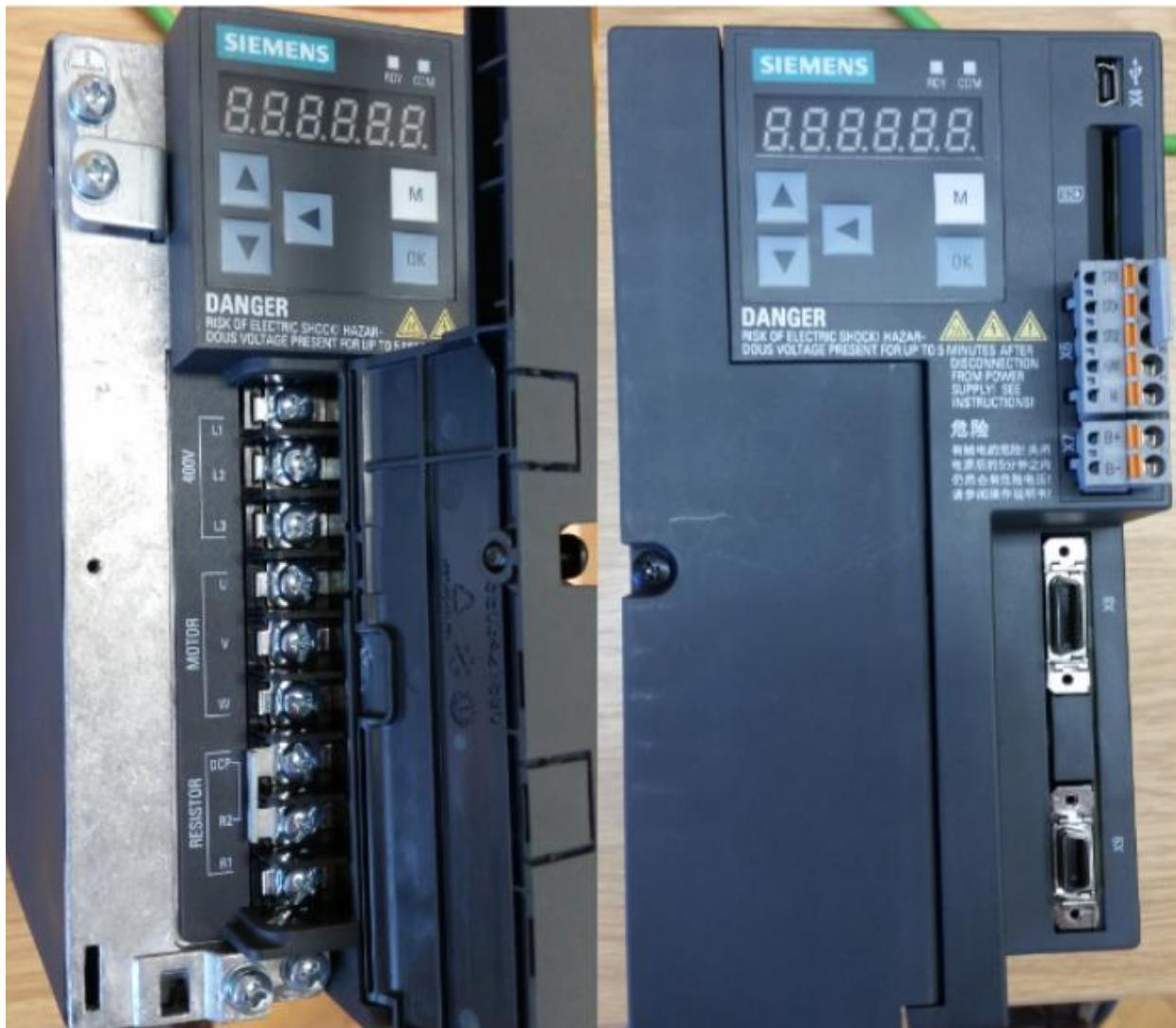
Slika 4.6 Siemens SINAMICS V90 servo driver
