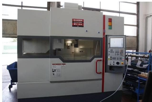
Slika 3.5 Glodalica Quaser mv184e
