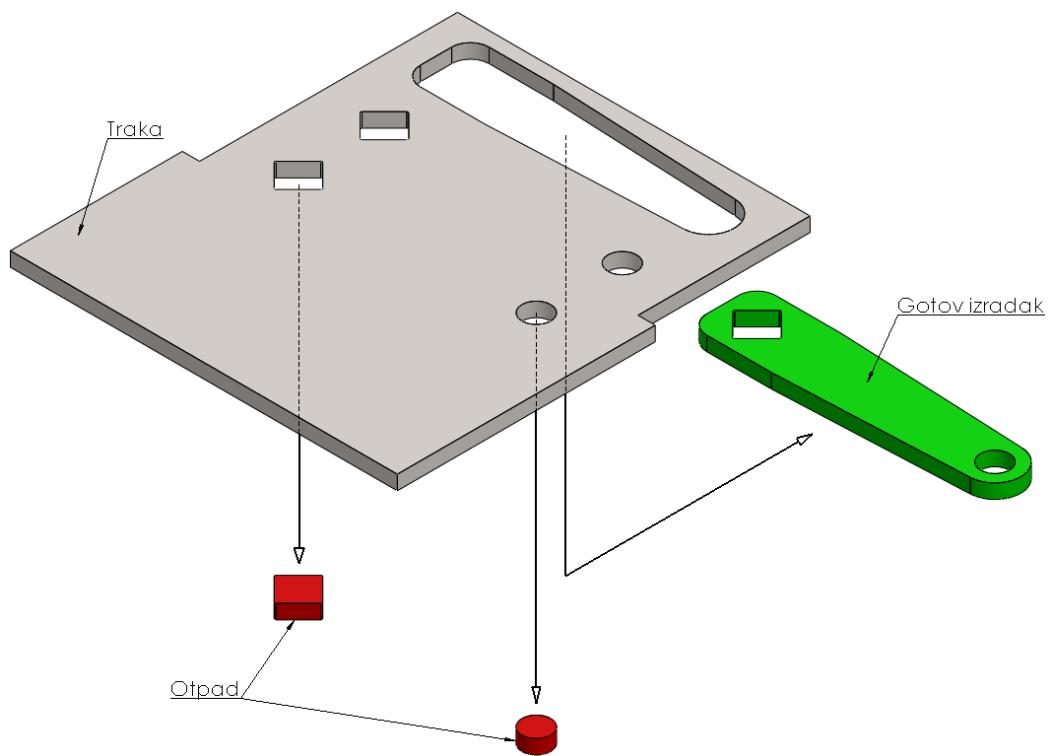
Slika 6.4 3D model trake
