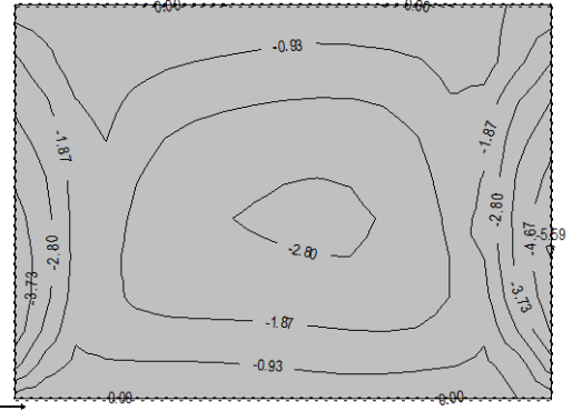
Okvir: V_3 Aa - g.zona - Pramac 1 - max Aa1,g= -5.59 cm²/m
