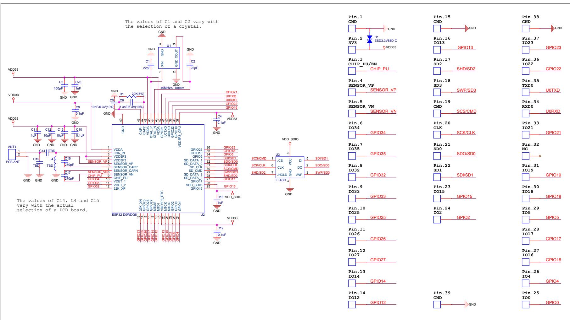
**Figure 3: ESP32-WROOM-32 Schematics**
