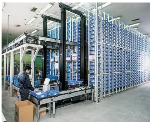
Slika 3.5 Micro-load AS/RS i Mini-load AS/RS [13]
