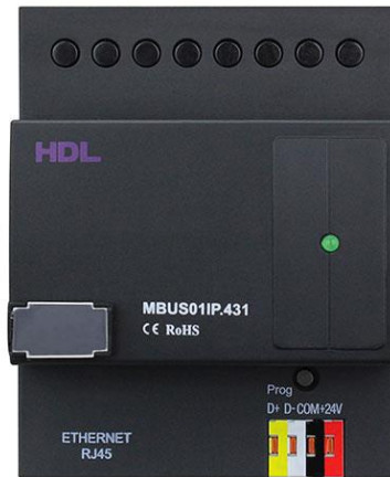
Slika 2.13. 1 Port Programming Gateway [19]
