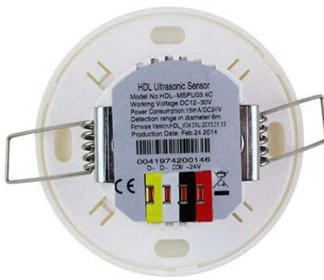
Slika 2.14. Ceiling Mount Ultrasonic Sensor [20]
