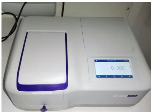
Slika 12: Spektrofotometar, UV/Visible Spectrophotometer 195-1050 nm, 4 nm bandwidth,
