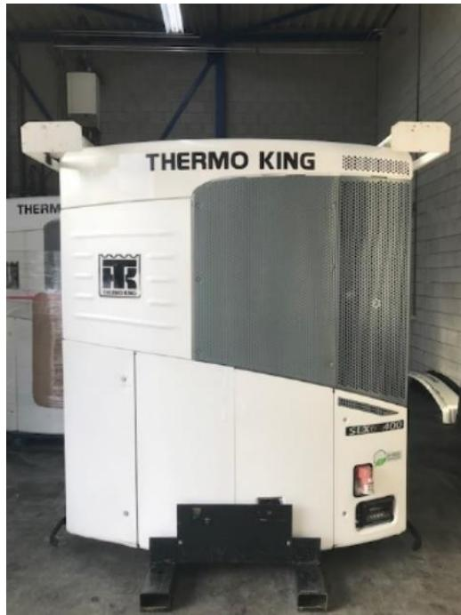
Slika 23: Rashladni agregat SLXi -400
