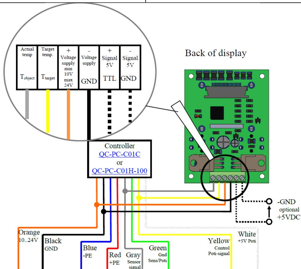
Slika 4.4 Shema spajanja displaya s regulatorom temperature [30]
