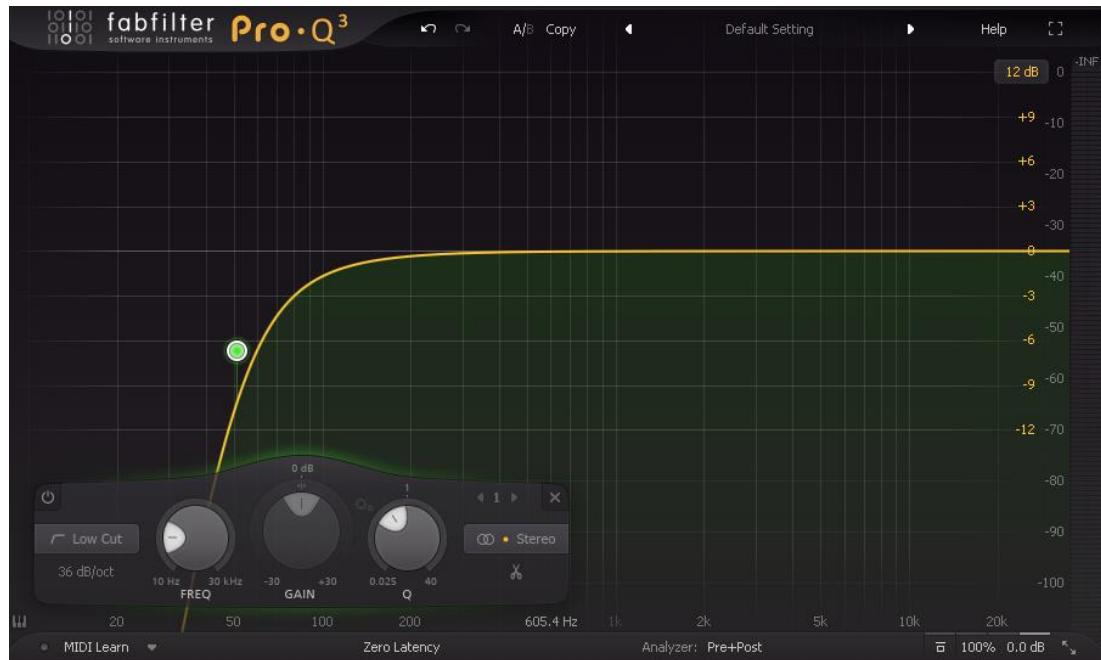
Slika 14. Fabfilter Q3 -Visokopropusni filter
