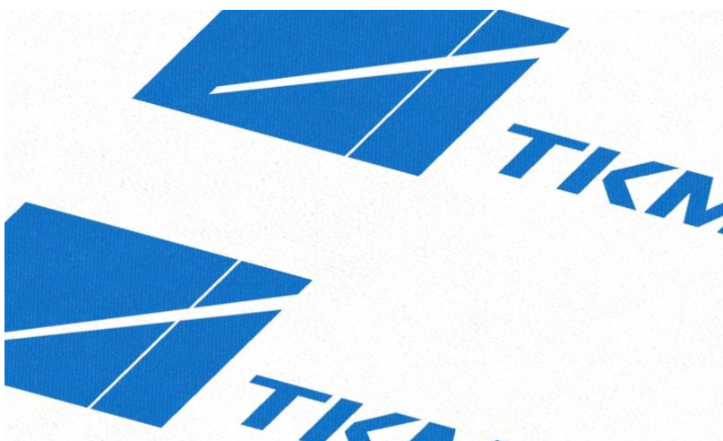
Slika 41. Negative doctor blade lines
