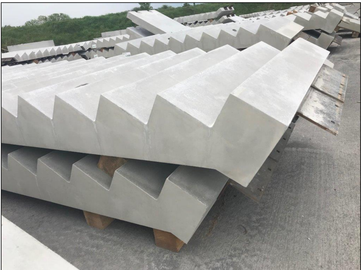
Slika 34: Odlaganje prefabriciranih stubišnih krakova (izvor: https://floodprecast.co.uk/2020/01/benefits-of-using-precast-stairs-with-steel-frame-buildings/ )
