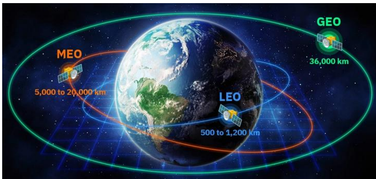
Slika 2.1. Prikaz osnovnih orbita satelita [ https://eos.com/blog/satellite-constellation/ ]
