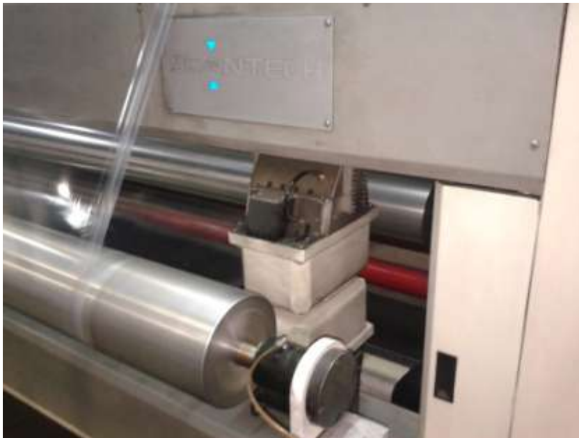
4.5 Scantech-ov rendgenski skener [25]
