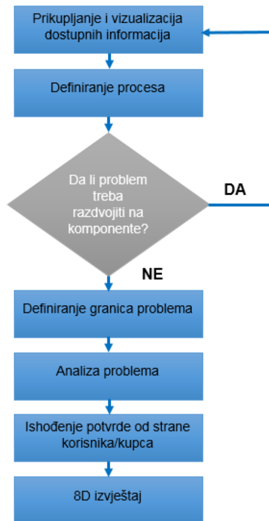
Slika 2.4.1. Definiranje problema (Izvor: Izradio autor. Prema: Begley Schade, Martha. 2013. 8D Problem Solving Process. Business Online Learning. Str. 40)
