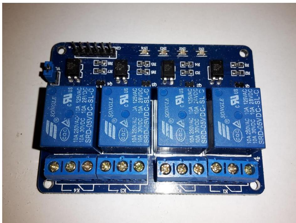
Slika 6.6 Modul sa 4 releja – Songle 4 Channel Relay Module 8051, [10]
