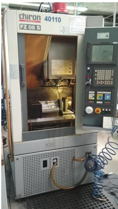
Slika 1.1. CNC glodalica Chiron FZ 08 S
