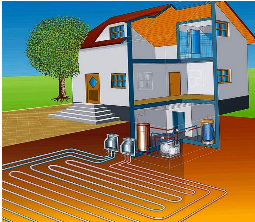
Slika 5 Sustav podzemnih toplinskih pumpi ( https://hr.vmat2.org/1499-how-to-make-a-heat-pump-for-home-heating-with-your-ow.html )
