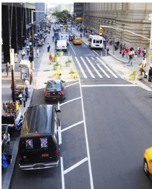
Slika 7.1.5. Produženi rubnici (Izvor: https://nacto.org/publication/urban-street-design-guide/street-design-elements/curb-extensions/ ;18.09.2019.)
