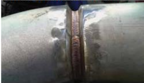
Tube welded with TETRA V 317L-G.
