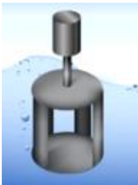
Slika 2.8. Squirrel cage Darrieus turbina [4]
