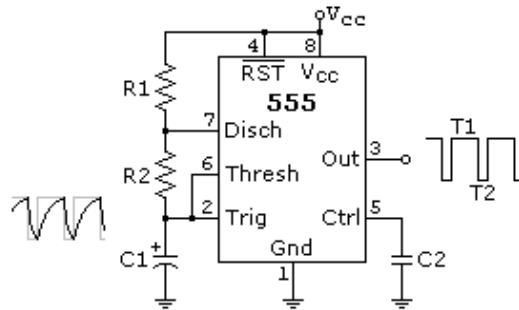
$$T_1 = \text{Time On} = 0.693 (R_1 + R_2) C_1$$
