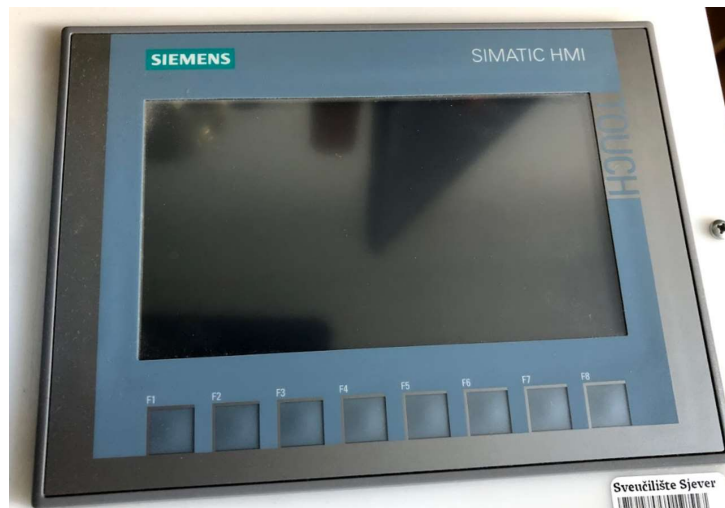
Slika 4. 2 Korišten HMI panel KTP700 Basic PN
