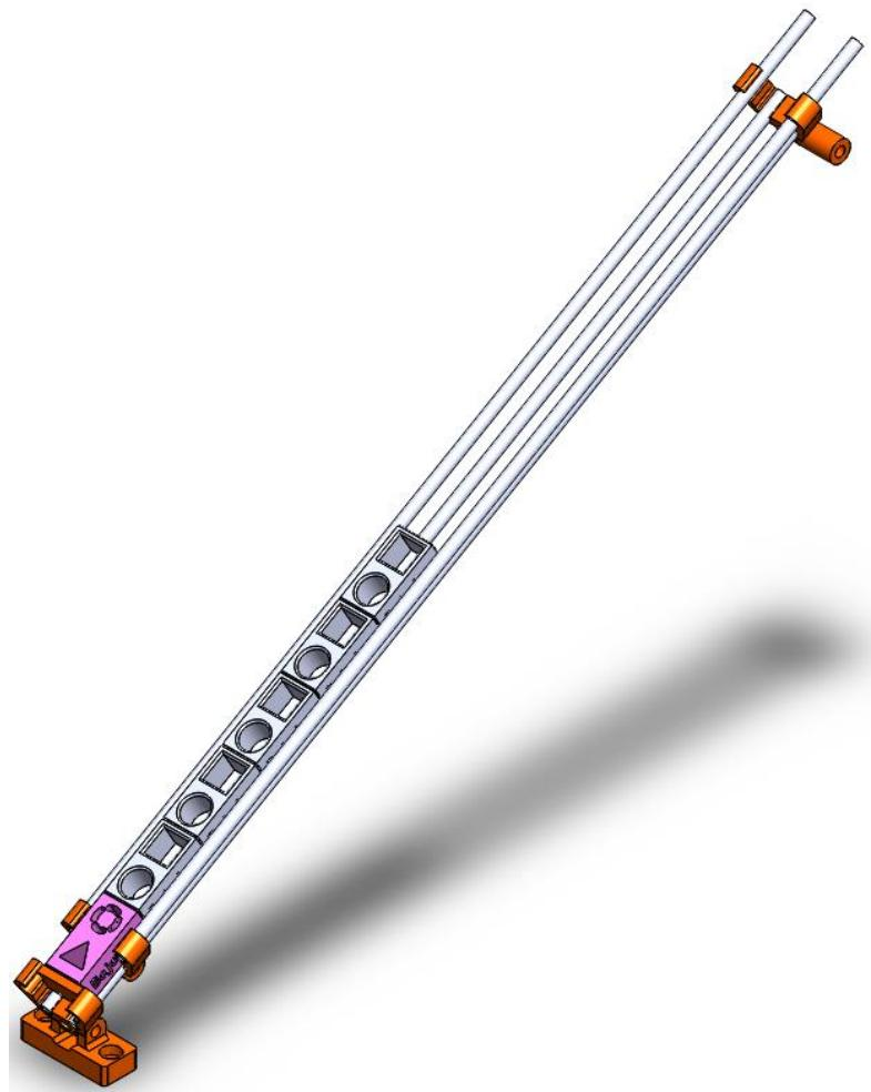
Slika 6.1 3D model klizne staze u SolidWorks-u
