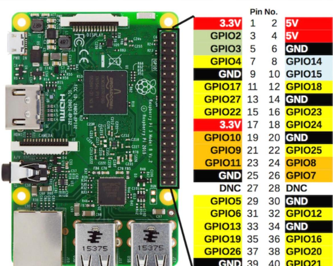
Slika 3.21 GPIO izlazi na RPI računalu, <https://www.bigmessowires.com/wp-content/uploads/2018/05/Raspberry-GPIO.jpg>
