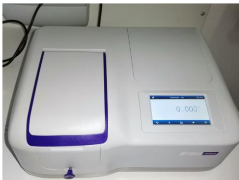
Slika 12: Spektrofotometar, UV/Visible Spectrophotometer 195-1050 nm, 4 nm bandwidth, Italija
