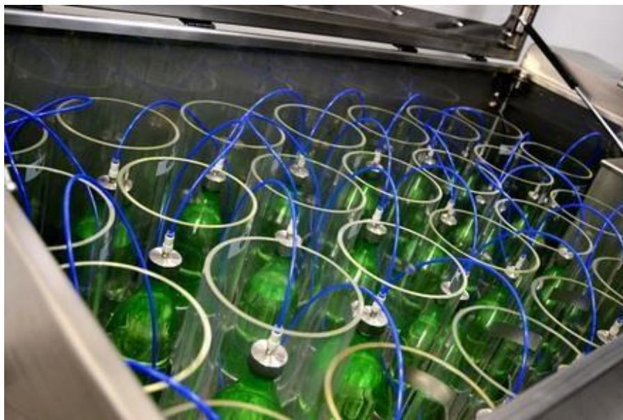
*Slika 13. Crack test PET boca [Izvor: Martin Božurić]*
