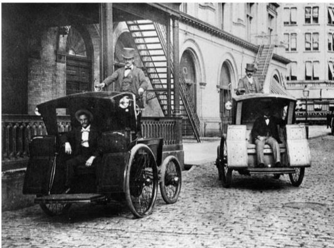
Morris and Salom Electrobats are seen in front of the Old Metropolitan Opera House on 39th Street in the Manhattan borough of New York, 1898. The electrobats were battery-powered cars that served as early taxis in the city.
