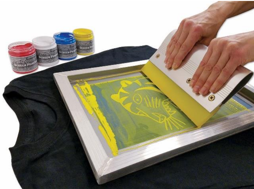
Slika 13 Sitotisak (izvor: https://images.squarespace-cdn.com/content/v1/5ac4eb022971149bb6d709d3/1549402246418-WXMAVB6NWN8KY0V3G9AP/JSI-Kits-screen-pull-dark-t-shirt )
