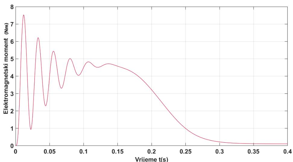
Slika 24: Model 3 – zalet, moment – motor 600 W
