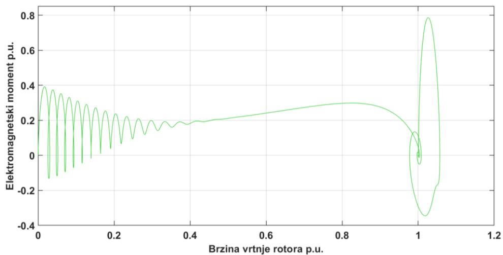
Slika 34: Model 2 – zalet Y-Δ, moment vs brzina rotora – motor 600 W
