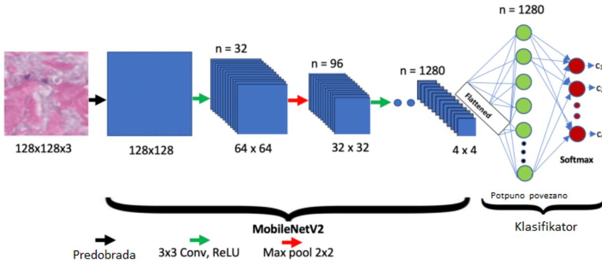
Slika 4.7 Arhitektura MobileNetV2 mreže (izvor. [https://www.researchgate.net/figure/The-proposed-MobileNetV2-network-architecture\\_fig1\\_350152088](https://www.researchgate.net/figure/The-proposed-MobileNetV2-network-architecture_fig1_350152088))
