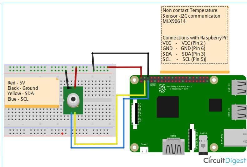
Slika 5.1 Shema spoja infracrvenog senzora sa Raspberry Pi računalom (izvor. <https://circuitdigest.com/microcontroller-projects/iot-based-contactless-body-temperature-monitoring-using-raspberry-pi-with-camera-and-email-alert>)
