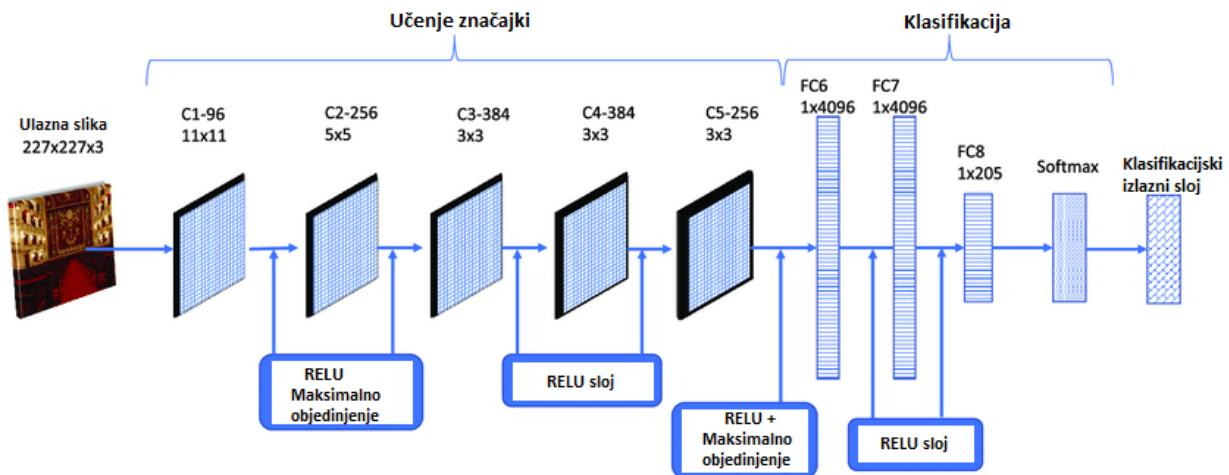
Slika 4.11. Konvolucijska neuronska mreža bazirana na Caffe modelu (izvor. [https://www.researchgate.net/figure/CNN-places-architecture-design-based-on-the-pre-trained-Caffe-model-Layers-fc7-and\\_fig1\\_332665758](https://www.researchgate.net/figure/CNN-places-architecture-design-based-on-the-pre-trained-Caffe-model-Layers-fc7-and_fig1_332665758))
