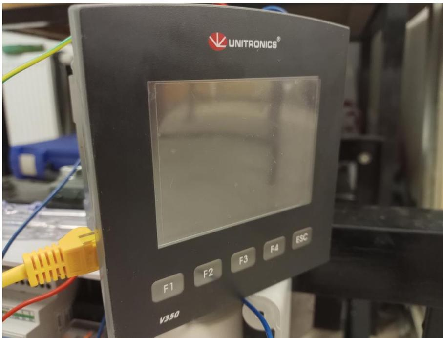
*Slika 4.1.1. Unitronics V350 PLC+HMI*
