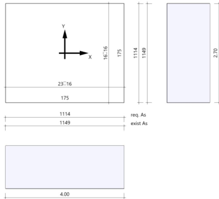
The peak values of the distribution according to Bulletin 240 of the German Committee for Reinforced Concrete will be covered. Therefore, the here required reinforcement may be higher than the required reinforcement. In order to ensure the transverse carrying capacity, the foundation has been dimensioned in the punching range for minimum moments according to equation (NA.6.54.1), provided the shear force determination has not led to higher values.
