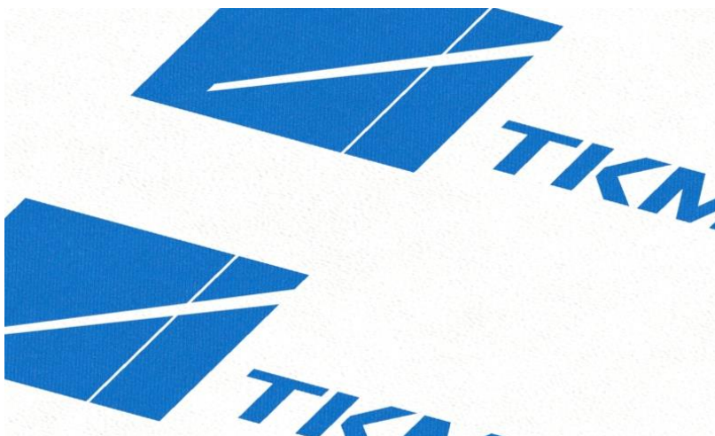
Slika 41. Negative doctor blade lines
