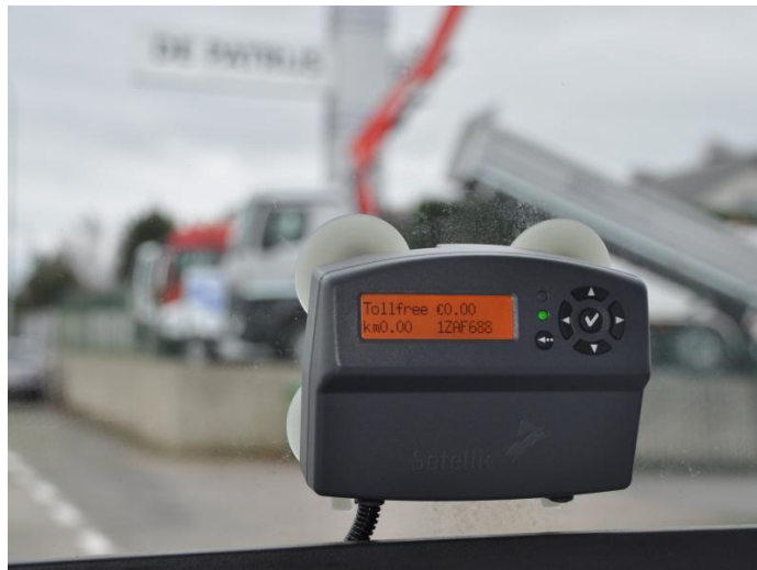
Slika 41 On Board Unit (OBU)
