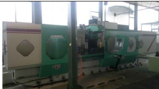
Slika 4.12 CNC brusilica Rosa – Linear Silver 30.8
