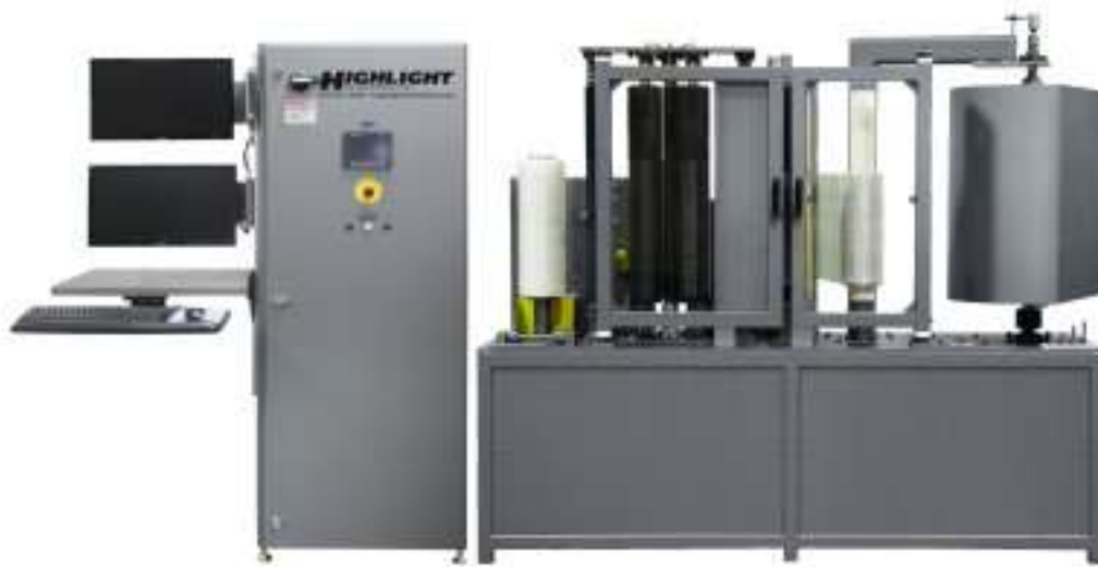
4.24 Highlight stretch film test stand [17]
