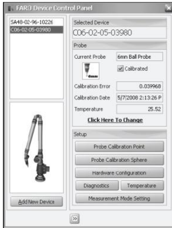
Slika 22. Control Panel FARO
