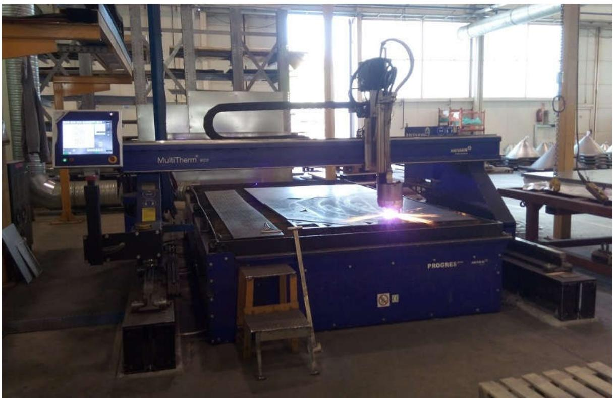
Slika 3.6 CNC plazma rezaca Hypertherm HPRXD 260 [27]
