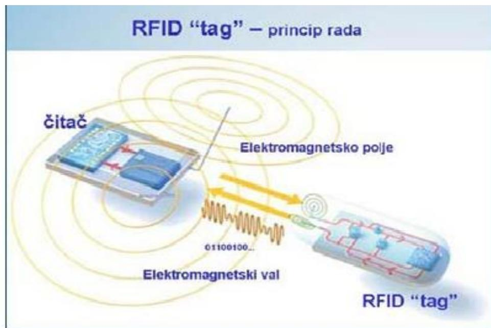
Slika 11.: RFID TAG – Radio frequency identification
