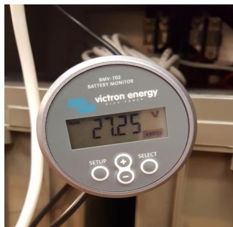
Slika 4.3 Victron Energy Battery Monitor BMV-702
