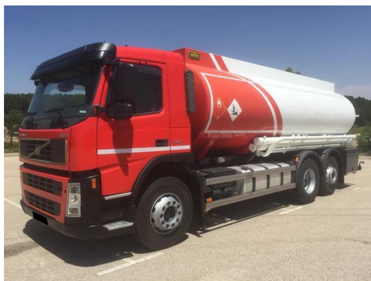
Slika 20: Prikaz cisterne integrirane na kamion sa oznakama opasnosti ( https://imgredirect.milanuncios.com/fg/2335/29/camiones-usados/Volvo-cisterna-20000litros-hidrocarburos-233529454_1.jpg?VersionId=liPd2bgXNcChryPLghTHTNImhnJa8pgE )
