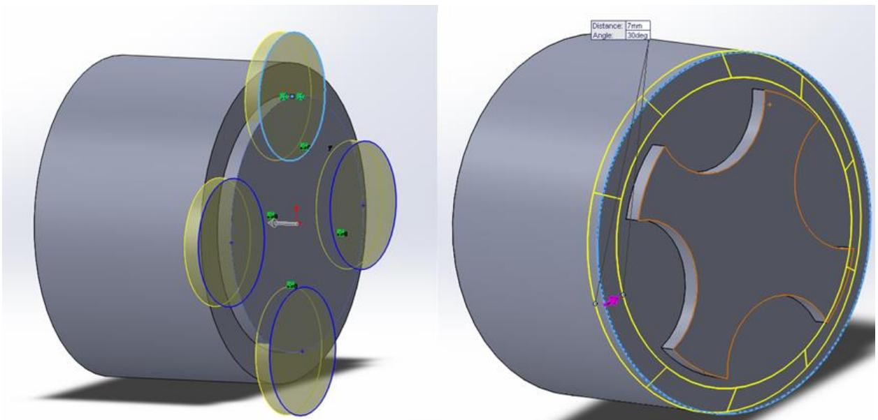
Slika 6.4 Naredbe Circular Pattern i Chamfer [20]
