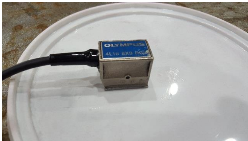
Slika 50: Sonda OLYMPUS 4L16-8X9-DGS1-P-2.5
