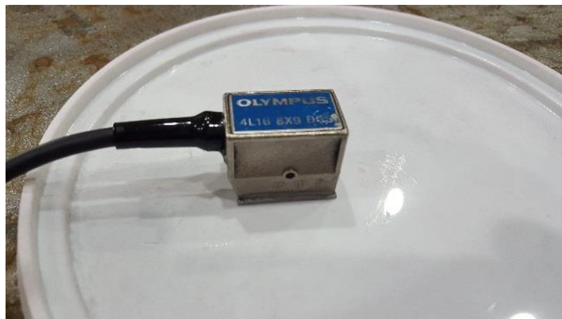
Slika 50: Sonda OLYMPUS 4L16-8X9-DGS1-P-2.5
