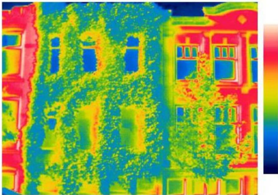
*Slika 4.2.1.2. Snimak pročelja infracrvenom kamerom (izvor: Perini K, Ottelé M, Fraaij A, Haas E, Raiteri R. Greening the building envelope, façade greening and living walls systems. Open J Ecol 2011;1: str.1–8.)*
