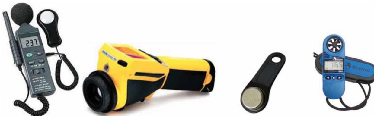
Slika 5.4.1. Uređaji korišteni u studiji: mjerач okoliša, iButton, termalni fotoaparati, anemometar (izvor: MaricruzSoleraJimenez (2018) Green walls: a sustainable approach to climate change, a case study of London, Architectural Science Review, 61:1-2, 48-57, str.:51)
