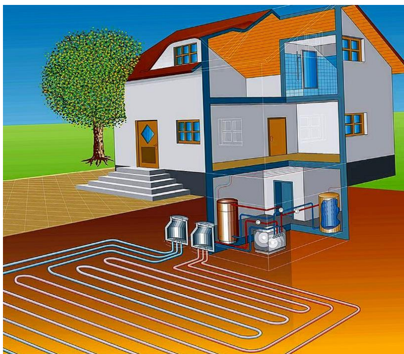
Slika 5 Sustav podzemnih toplinskih pumpi ( https://hr.vmat2.org/1499-how-to-make-a-heat-pump-for-home-heating-with-your-ow.html )
