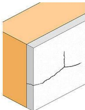
*Slika 2.5.3.1. Pukotine uslijed spuštanja (Izvor: <https://www.roefix.hr/O-nama/Aktualno/Novosti/Pukotine-na-fasadi>)*
